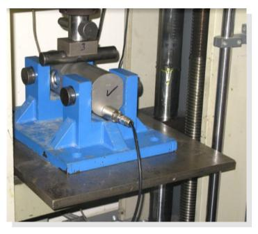
Close-up of Load Cell connection and stainless steel housing that contains the *Mantracourt D*-*Cell* microcomputer. The Load Cell Programmer can be connected direct to the load cell using the short cable with stainless steel connector
