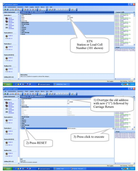
This should have changed the address; as a check, repeat the procedure using the new address of "1" at the opening screen to see it has been accepted.
