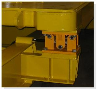
Load Cell complete with mounting cradle in-situ on Trailer Chassis
