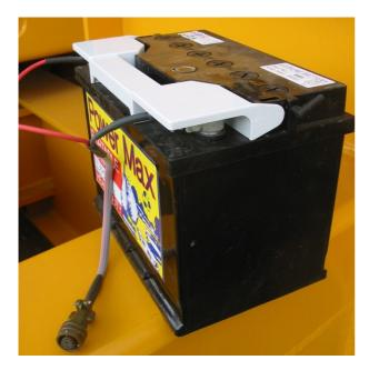
The cable from the Battery Pack includes an in-line *automotive* Fuse-Holder with 7.5Amp fuse fitted in the +ve feed (**RED Wire**) and a *MIL spec*, 2 way cable socket for connection to the trailer and the battery charger.
