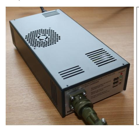
The connector on the front panel is a *MIL spec*, 2 way plug which will mate directly with the 2 way cable socket on the *Battery Pack* cable.
