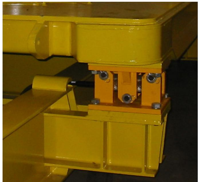
**N.B. It is good practice to periodically clean the load cells from any debris. Any build-up of detritus that affects the deflection of the load cell **will also affect the accuracy.****
