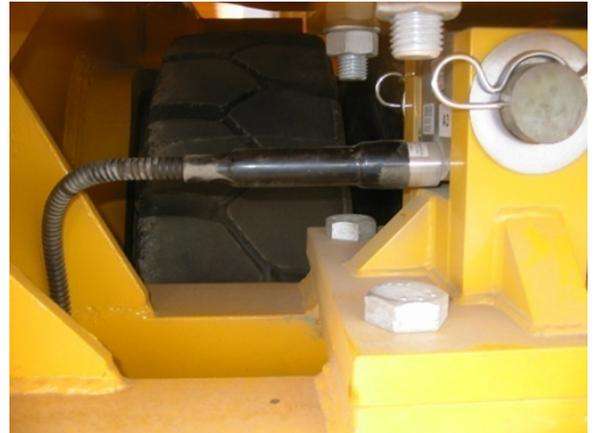
The earth point should be cleared of paint and as close as possible to the area being welded. If the area to be welded is on the weighing platform then the earth clamp should also be on the weighing platform and similarly with the main chassis. **If the earth clamp is fixed to the chassis whilst welding the weighing platform the current path will be through the load cell / load cells and they will be seriously damaged.**
