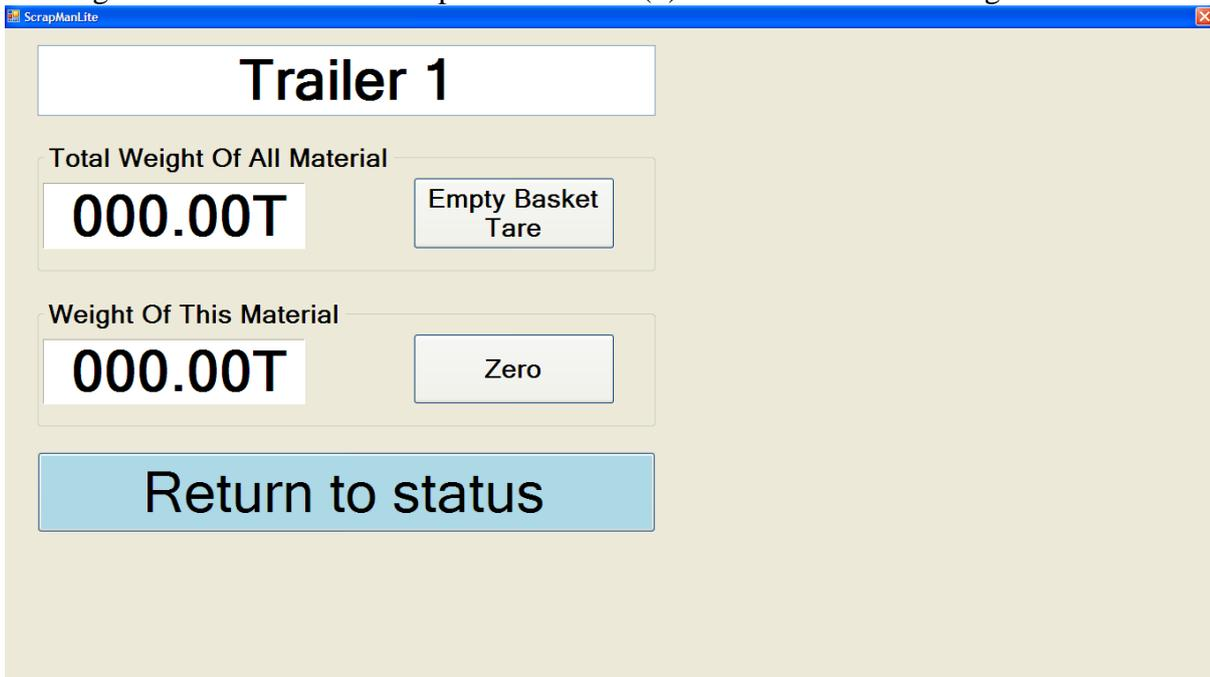
When a new, empty basket is put on the Car Frame it is important to do an 'Empty Basket Tare'. This will clear the 'total weight of all material' down to zero and be ready for loading. There is a warning to give you chance to change your mind; you would normally press 'Yes'.
