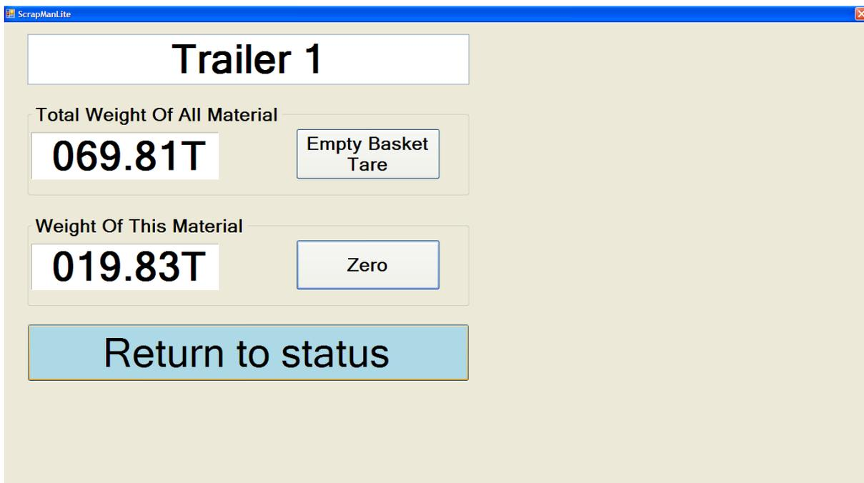
In this case, a further 20T has been loaded to the basket making the Total Weight 70T
