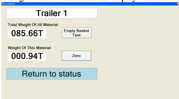
The ACTUAL LOAD Reading of 0.94T is written on the recipe and the Zero button is pressed showingí .
