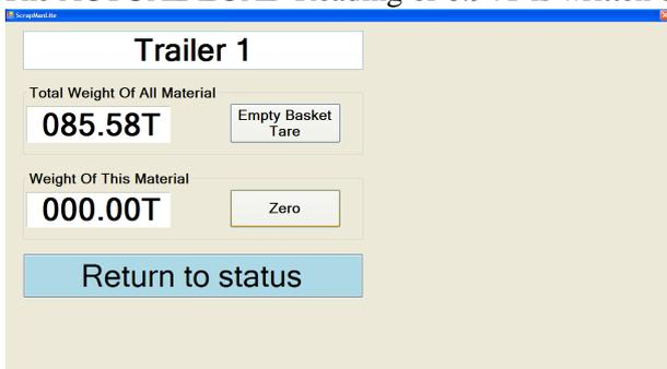
The Fifth (Final) material *Lime* is loaded until the *Weight Of This Material* is approx equal to the required tonnage of 2.00 Tonnes and the display will showí .
