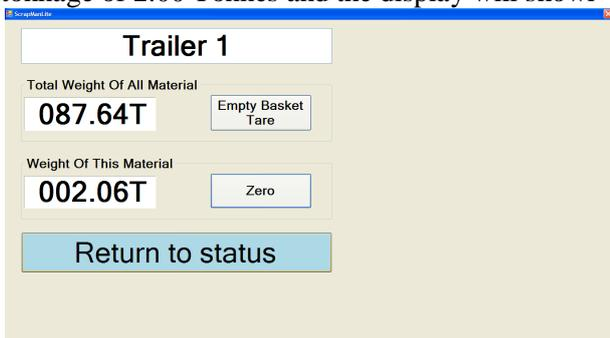
The ACTUAL LOAD Reading of 2.06T is written on the recipe and the cycle is complete
