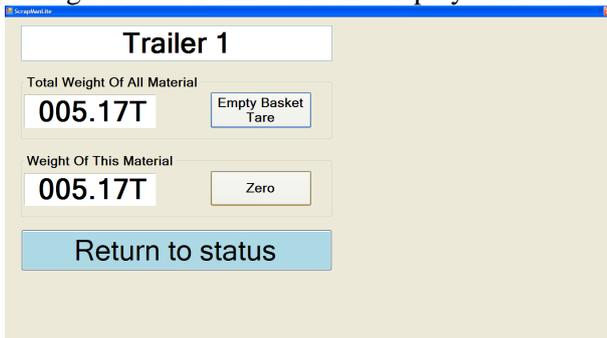
The ACTUAL LOAD Reading of 5.17T is written on the recipe and the Zero button is pressed showing:
